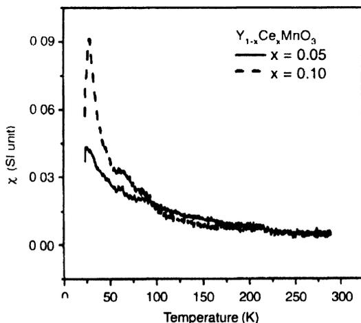
Figure 6. Temperature variation of inphase susceptibility ( $\chi'$ ) of  $Y_{1-x}Ce_xMnO_3$  samples for  $x = 0.05$  and  $0.10$ .
