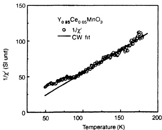
Figure 7.  $1/\chi'$  versus Temperature for the sample  $Y_{0.95}Ce_{0.05}MnO_3$ . Solid line represents the fit to the Curie-Weiss law.
