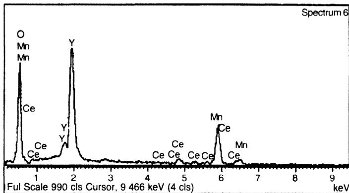
Figure 5. Typical SEM-EDS spectra for  $Y_{0.9}Ce_{0.1}MnO_3$  sample
