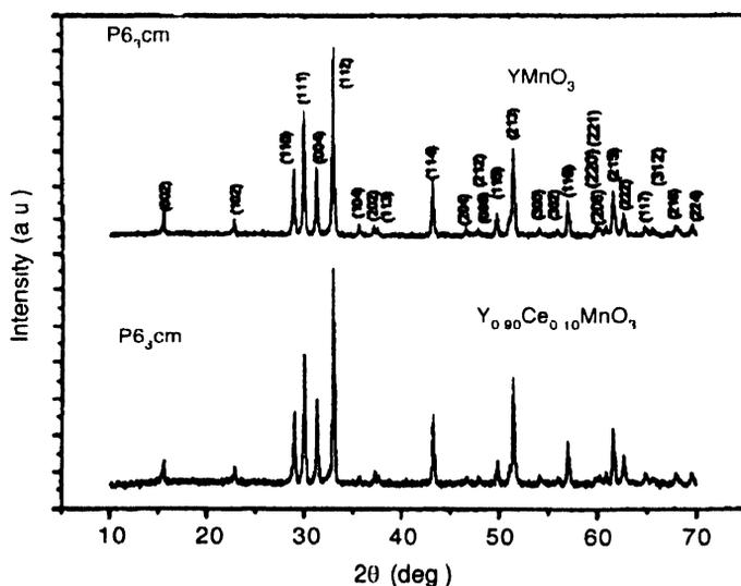
Figure 1. XRD patterns of  $\text{YMnO}_3$  and  $\text{Y}_{0.9}\text{Ce}_{0.1}\text{MnO}_3$
